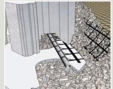
**It's Versatile...** Variable setbacks, sharp radius turns, "One Unit" construction, and complete interchangeability are all features of Rockwood's Classic System. The ability to mix various sizes and colors within a wall enhances your imagination without sacrificing structural integrity. Plus, the Anchor Bar allows you to build at any setback you desire – from 0° to 14°, providing the only "true" vertical setback in the industry.
